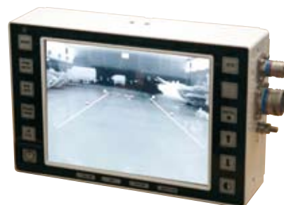
Driver Display Unit dimensions (mm) Width 248mm, Height 160mm, and Depth 66mm
